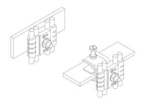
Through popular demand GCA Ltd produced the 4 way clamps to reduce costs of purchasing 2 doubles, with longer studding etc. Both clamps will hold single or double cables adequately allowing additional cable to be easily added later. All two piece 4 way clamps are designed to precisely fit the cable diameter. All 4 way clamps externally interlock with single and double clamps.
