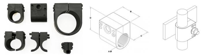
All two piece single clamps are designed to precisely fit the cable diameter. A range of 11 cable diameters from 5mm to 58mm are available. All single clamps externally interlock with double and 4 way clamps. These GCA Ltd single clamps are manufactured in high grade polypropylene and UV: stabilised to prevent degradation or breaking. For 'flame retardant' clamps to UL94V-0 (0.8mm) LSF Halogen and Phosperous free material state 'BW4-5/8"FR'.
