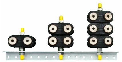
Length of M10 stainless steel threaded studding required for stacking: - single, two or three double or single GCA Ltd clamps, using a maximum 3 x M10 s/s Full Hexagon Nuts, 4 x M10 s/s Form 'B' Flat washers, and 2 x M10 s/s SQ Section Spring Coil Washers. N.B We have allowed additional 4mm for steel work and approx. 15mm maximum – studding protruding after tightening of clamps.
