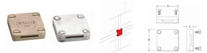
These four-way connectors are suitable for making cross, straight through or tee joints in flat tape. The base has a countersunk hole in the middle of securing the clamp to the building surface and the lid is fixed by means of four screws.
