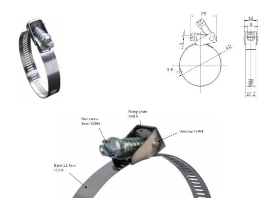
Quick release style worm drive clips are indispensable for installation in closed systems where the clamp must be disengaged to be applied. The swivel-action locking of screw to band makes both installation and removal fast and easy.
