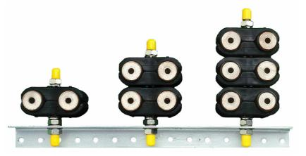
Length of M10 stainless steel threaded studding required for stacking: - single, two or three double or single GCA Ltd clamps, using a maximum 3 x M10 s/s Full Hexagon Nuts, 4 x M10 s/s Form 'B' Flat washers, and 2 x M10 s/s SQ Section Spring Coil Washers. N.B We have allowed additional 4mm for steel work and approx. 15mm maximum – studding protruding after tightening of clamps.
