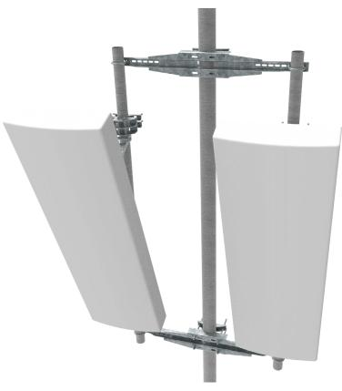
Designed to provide support for two heavy antennas offset symmetrically from a central parent pole. The double parent pole clamp eliminates rotational slip even if the bracket is asymmetrically loaded.
