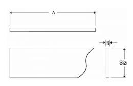
PVC covered aluminium tapes are available in a choice of six standard colours to match the most common building materials and provide an aesthetic finish to the external lightning protection system. All PVC coverings are UV stablished although some discolouration may occur over time.
